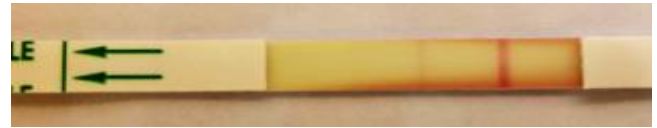
Figure 5. Detection of CPS in macaque urine. Urine sample was collected at day 4 post B. pseudomallei infection. Sample was diluted 1:1 in chase buffer and tested on the 3C5 AMD LFI.
